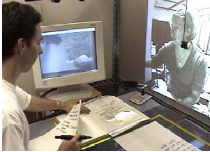
Figure 6. Projection of remote person's hand gesture
